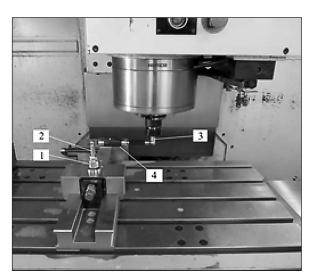
Fig. 1. Measuring device Ballbar QC20: 1 – Magnetic center holder, 2 – Magnetic centre cup attached to rack, 3 – Magnetic centre cup clamped in collet, 4 – Measuring device
